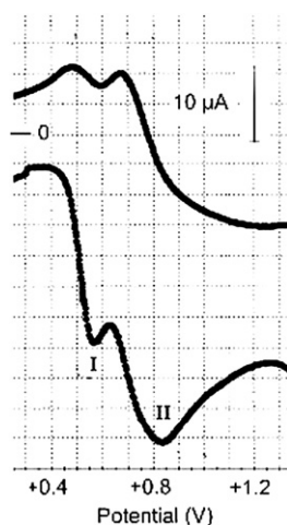
Figure 7. CVs of a 2.0 mM 4 + \text{K}^+ solution in 0.10 M \text{Bu}_4\text{NPF}_6/\text{MeCN} . Potential scan rate 100 mV/s.
